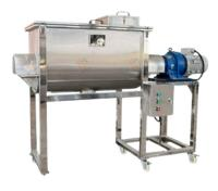
Ribbon blender are equipment used for mixing powder and granular based products thoroughly with the help of helical ribbon type blade.
