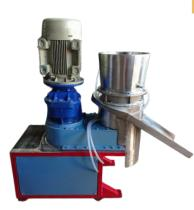
Basket Extruder is a machine widely used to get extrudes from wet mass.
